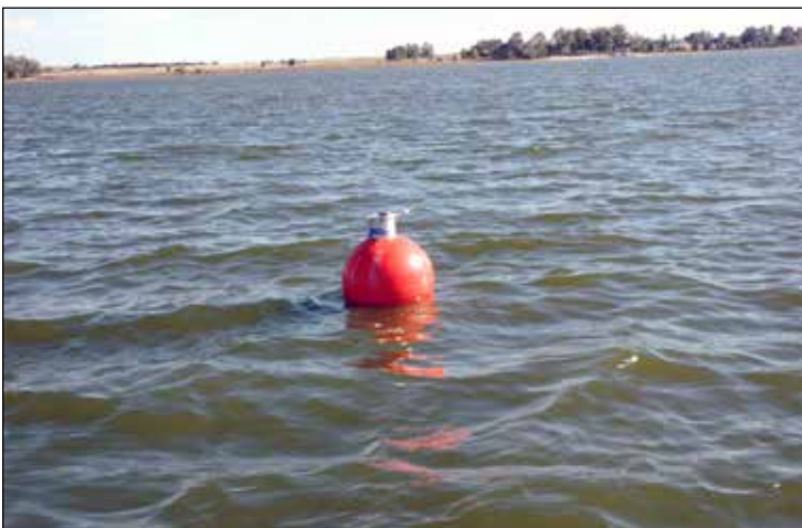
Long-term deployment buoy with telemetry. Monitoring equipment are fixed at 1-meter and about 8-meter depths to collect data every 30 minutes. The data is uploaded to a website every 12 hours.
