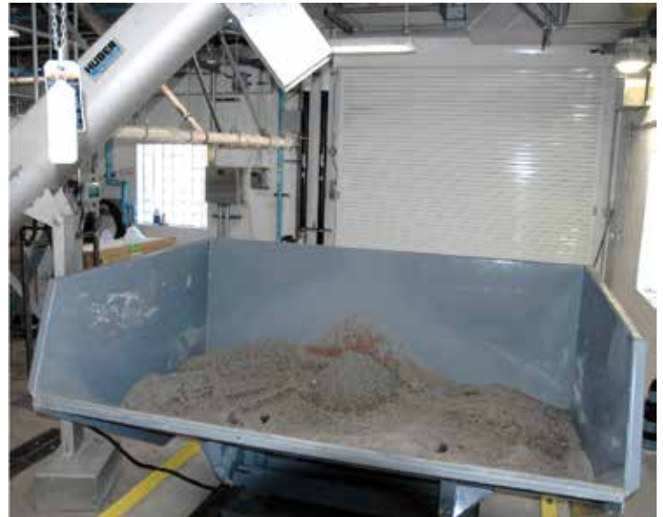
Phosphorus recovery dropping into a bin at a wastewater treatment plant that serves 2.2 million people. This phosphorus will be repurposed instead of sent down river.
