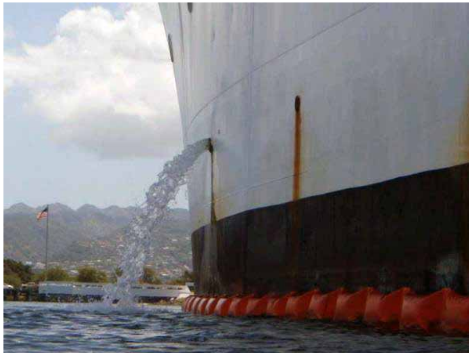
Figure 2. Ballast water being discharged from a vessel.
