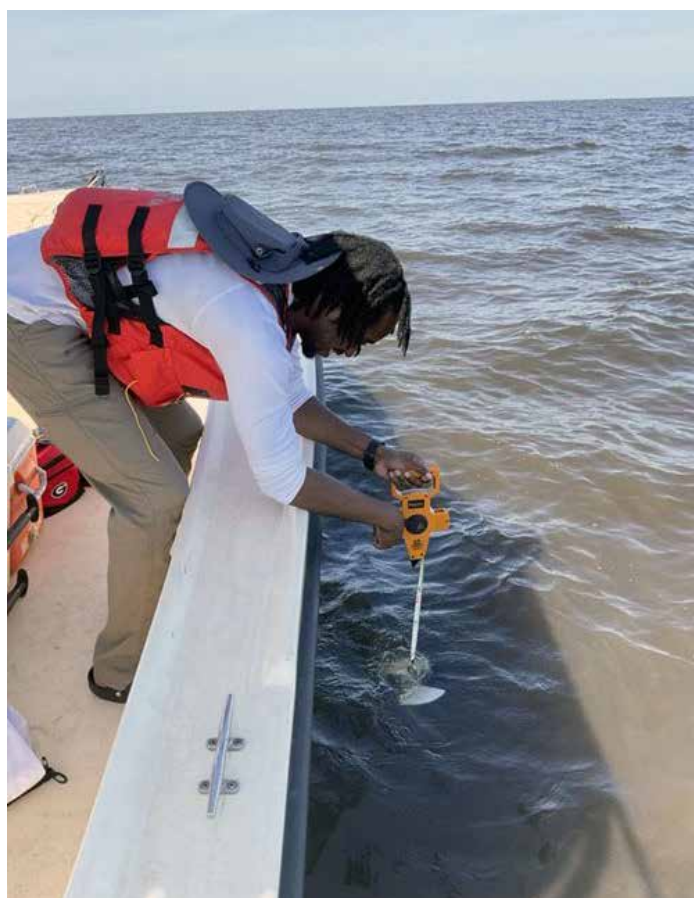
Figure 6. EPA Region 4 crew member lowering a Secchi disk to assess water clarity in Lake Okeechobee.
