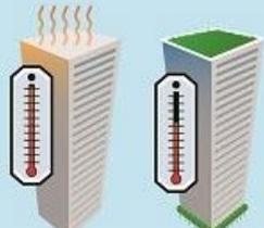
Studies show that green roofs can **reduce the energy** needed for cooling on the floor below the roof by more than **50%**<sup>5</sup>
