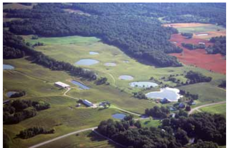
Figure 11. Area of potential karst and karst lakes. Left panel: Distribution of carbonate rocks susceptible to karst in the Great Lakes states (geology from Tobin and Weary 2004). Location of the photograph is shown as the pink box. Right panel: Low-angle oblique photograph of karst ponds about 5 miles west of Waterloo, Illinois (see Figure 1 for location). A veneer of glacial sediment covers the landscape and the sinkholes in the karst landscape. Viewpoint is from southwest to northeast. Photograph by Joel Dexter. ©2012 University of Illinois Board of Trustees; used courtesy of the Illinois State Geological Survey.
