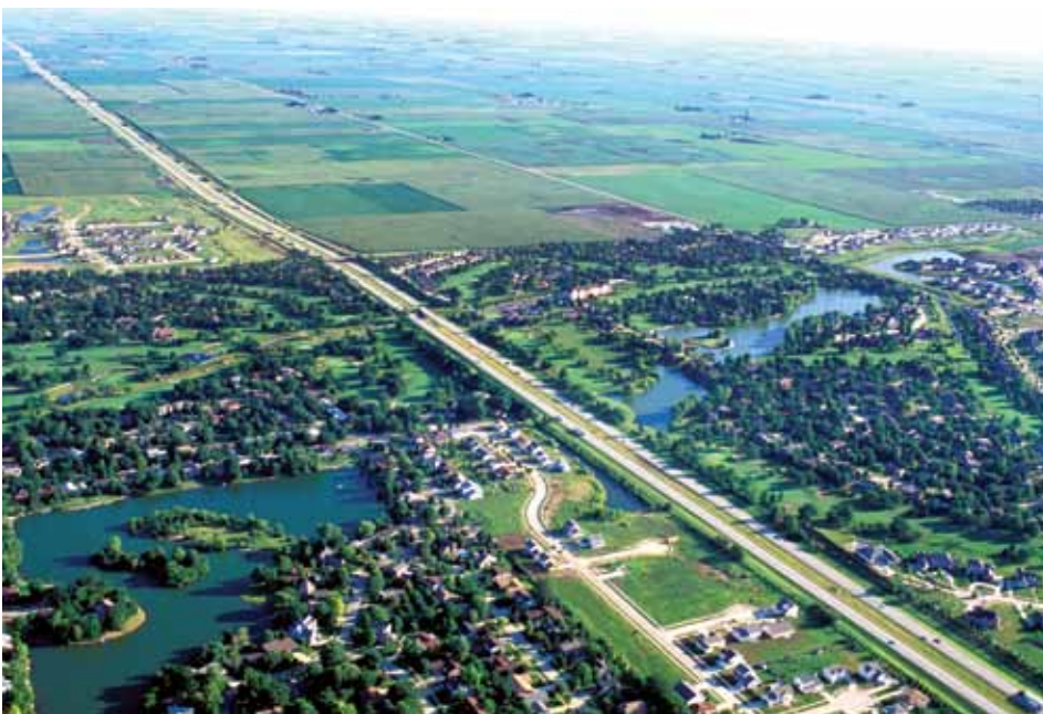
Figure 12. Human-made urban lakes are built to capture storm water runoff and add aesthetic value for home owners. Upper panel: Shaded relief image map of a part of the City of Champaign, Illinois. Lower panel: Low-angle oblique photo of southwest Champaign, Illinois. Suburban development straddles Interstate 57. Viewpoint is from northeast to southwest. Photograph by Joel Dexter. ©2012 University of Illinois Board of Trustees; used courtesy of the Illinois State Geological Survey.
