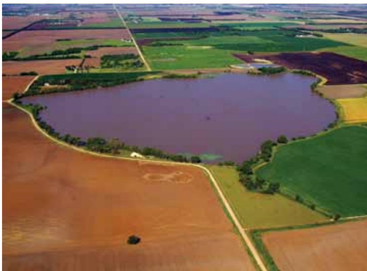
Figure 17. Inman Lake located south of Goveland, Kansas (McPherson Co.) occupies an undrained depression covering about 160 acres. This depression or sinkhole was caused by salt dissolution and resulting subsidence of the land surface. Photograph courtesy of Bill Johnson.
