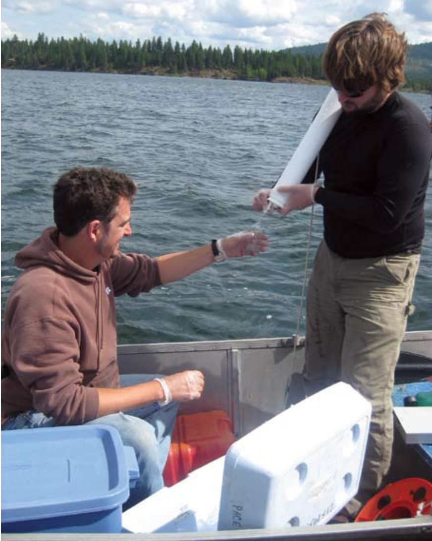
Figure 9. Dr. Marc Beutel and doctoral student Stephen Dent collect water samples for analysis of trace levels of total mercury and methylmercury. A number of strategies were used to minimize the potential for contamination, including the use of a Teflon water sampler; bottles that undergo a rigorous cleaning protocol, and the use of the clean hands-dirty hands technique in which the bottle holder touches nothing but clean bottles.
