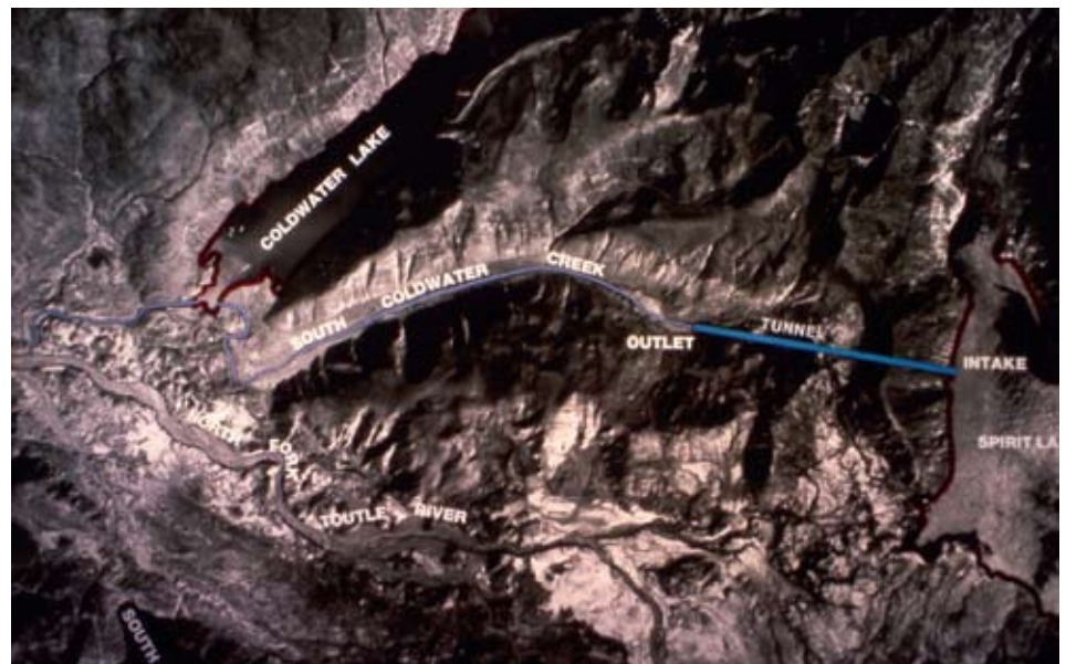
Figure 7. Map of the Spirit Lake tunnel outlet. The tunnel, 2.6 kilometers in length and 3.4 meters in diameter, was constructed between June 1984 and April 1985 at a cost of about $14 million. The tunnel extends under Harry's Ridge, the summit of which is at elevation 1,463 meters (above msl), or about 400 meters above the surface of Spirit Lake. Source: U.S. Army Corps of Engineers.
