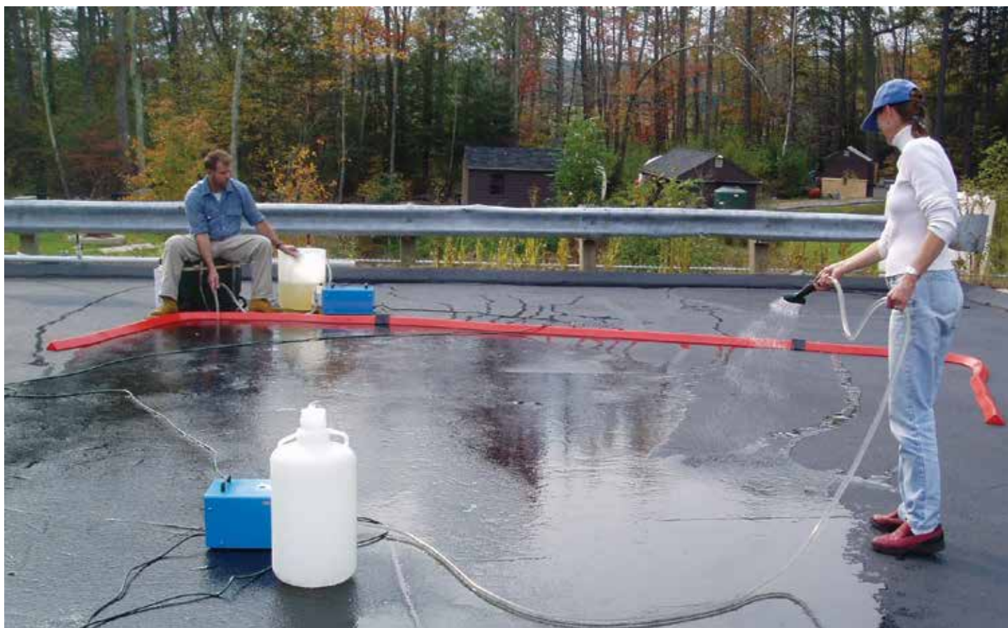
Figure 5. Researchers at the University of New Hampshire Stormwater Center simulate runoff on coal-tar-sealed pavement for measurement of polycyclic aromatic hydrocarbons (PAHs). Photo by the University of New Hampshire Stormwater Center.
