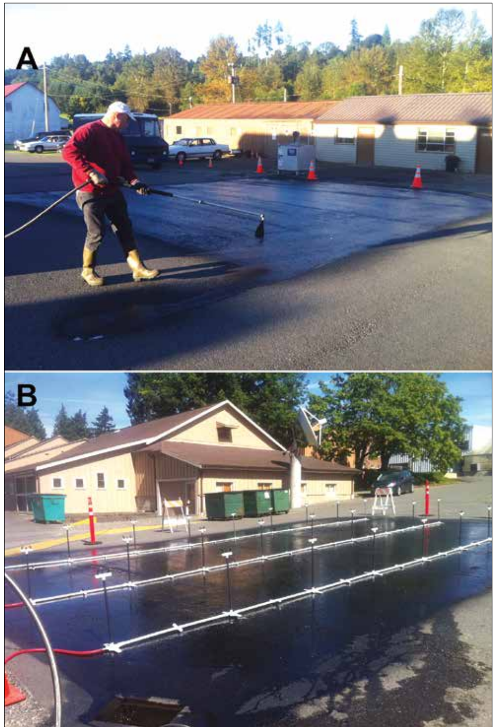
Figure 1. Coal-tar sealant application (A) and a sprinkler system to simulate rain on coal-tar-sealed pavement at Washington State University (B).
