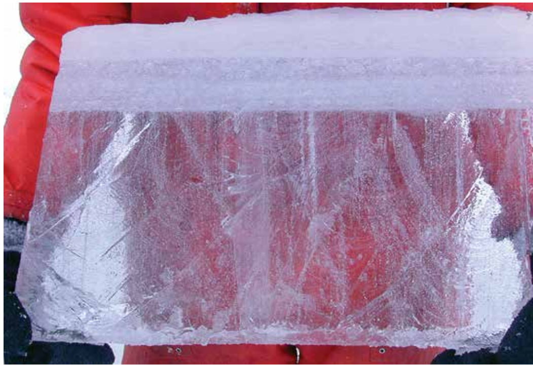
Figure 2. Vertical section of lake ice showing grey ice from frozen slush at top and clear ice below – Trout Lake, Vilas County WI, Feb. 2000. Small bubbles in clear ice are likely from dissolved gases in the water that were extruded as the water froze. Photo: Carl J. Bowser.
