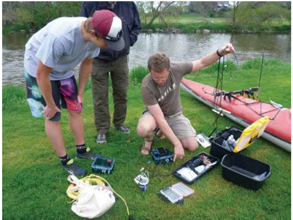
Figure 2. Monitoring the Rock River by Kayak – Professor Eric Compass, UW-Whitewater, and board member of the Rock River Coalition, led a kayak expedition the entire length of the Rock River. Samples of D.O., temperature, pH, and conductivity were taken every 10 seconds, and uploaded to a live feed. Photo by Lisa Conley.
